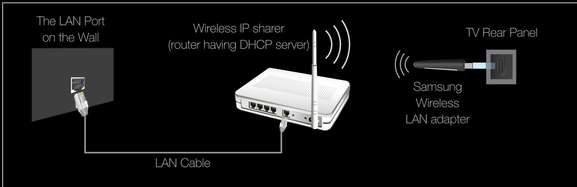
Samsung's Wireless LAN adapter is sold separately and is offered by selected retailers, Ecommerce sites and Samsungparts.com. Samsung's Wireless LAN adapter supports the IEEE 802.11a/b/g and n communication protocols. Samsung recommends using IEEE 802.11n. When you play video over a IEEE 802.11b/g connection, the video may not play smoothly.
