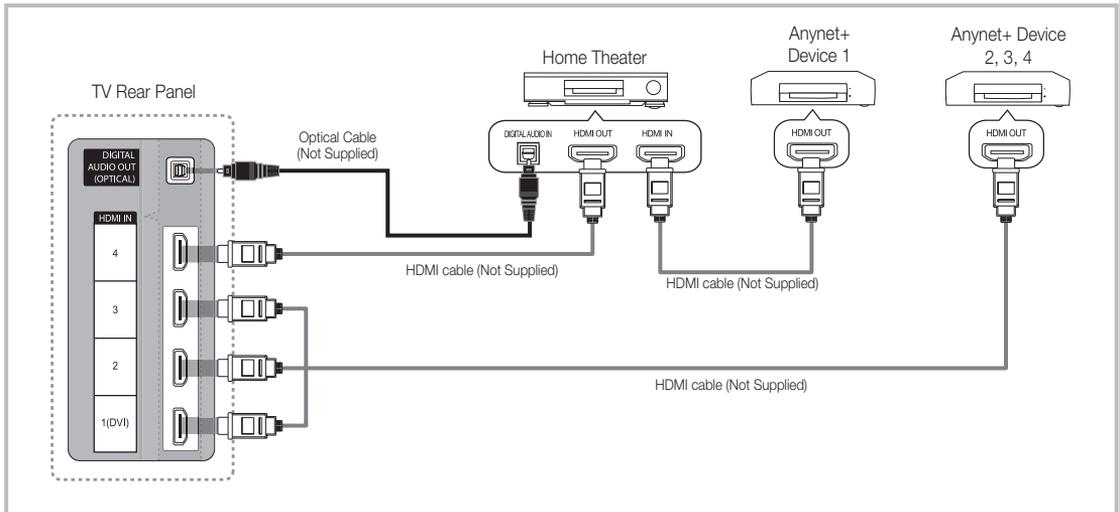
1. Connect the HDMI IN (1 (DVI), 2, 3 or 4) jack on the TV and the HDMI OUT jack of the corresponding Anynet+ device using an HDMI cable.
