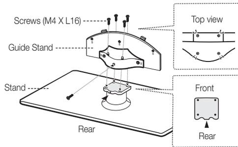
1. Connect the Guide Stand to the Stand using five screws (M4 X L16) as shown.
