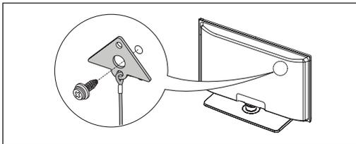
2. Firmly fasten the screw you provided (size M4xL20 or similar) to the wall or cabinet where the TV is to be installed.
