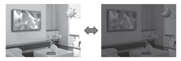
Eco Sensor measures the light in your room and optimizes the brightness of the TV automatically to reduce power consumption. This causes the TV to brighten and dim automatically. If you want to turn this function off, go to **Menu** > **System** > **Eco Solution** > **Eco Sensor**
