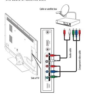
**4** Connect an audio cable (included) to the **L** and **R** audio jacks on the side of your TV and to the audio out jack on the cable or satellite TV box.
