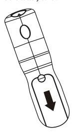
2 Insert two AA batteries into the battery compartment. Make sure that you match the + and – symbols on the batteries with the + and – symbols in the battery compartment.
