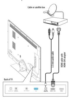
5 Connect a 3.5 mm audio cable (not included) to the PC/DVI AUDIO IN jack on the back of your TV and to the AUDIO OUT jack on the cable or satellite box.
