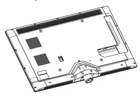
**2** Secure the stand to the screen with the four provided screws.
