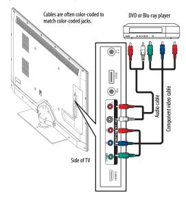
3 Connect an audio cable to the L/R (audio in) jacks on the side of your TV and to the L/R AUDIO OUT jacks on the component video device.
