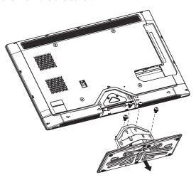
3 Secure the flat stand cover to the back of your TV using the four screws you just removed.
