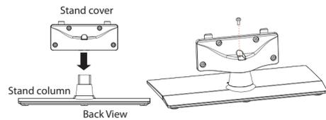
4 Secure the stand cover to the TV screen using four M5 x 12 mm screws (provided).
