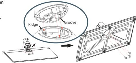
3 Align the stand cover with the stand column, then secure the stand cover to the stand column with one M5 x 12 mm screw (provided). Make sure that the bottom of the stand cover is flush against the top of the stand column.
